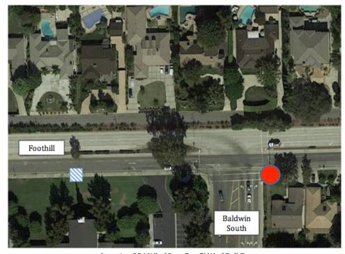
Location 224 W' of Stop Bar, 5' W of Pull Box Power is through existing conduit to controller cabinet Communication through existing conduit to controller cabinet
