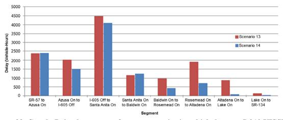
Figure 29. Graph. Delay by segment for two scenarios in vehicle-hours—I-210 VISSIM simulation.
