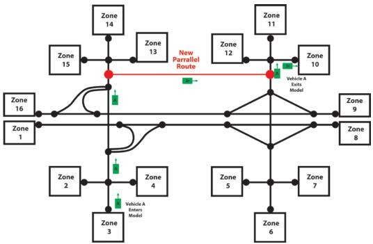
Figure 13. Illustration. O-D parallel facilities.
