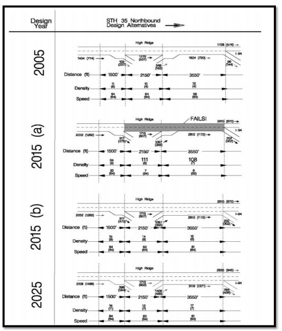
Figure 28. Illustration. Sample comparison of project alternatives using schematic drawing.<sup>(7)</sup>
