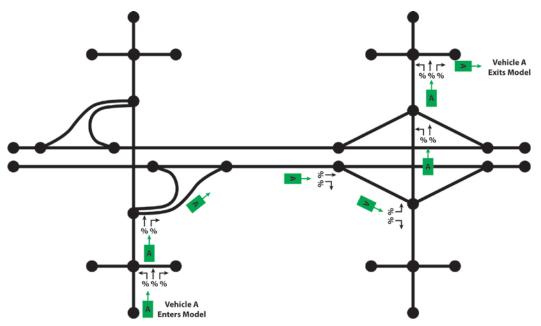
Figure 10. Illustration. Turn percentage O-D-based approach.
