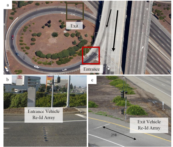
Fig. 1. (a) Hegenberger on-ramp entrance and exit. (b) Entrance Vehicle Re-Id Array. (c) Exit Vehicle Re-Id Array.
