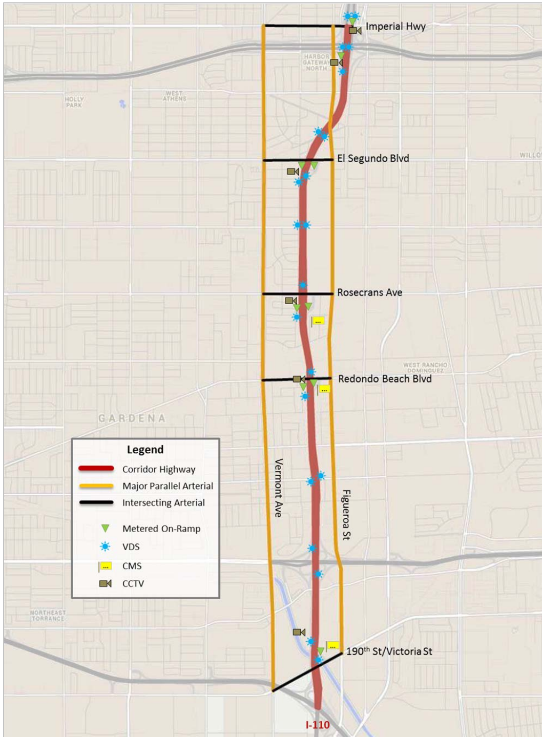
Figure 10. Corridor 2-B (I-110 North) Overview
