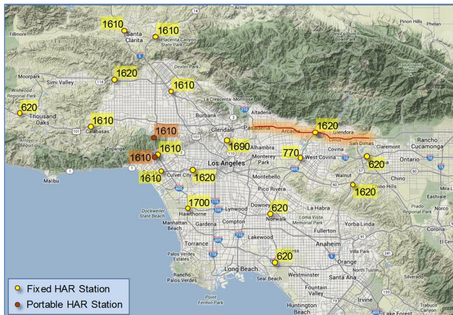
Figure 54 – Location and Broadcast Frequency of Highway Advisory Radios in Caltrans District 7
