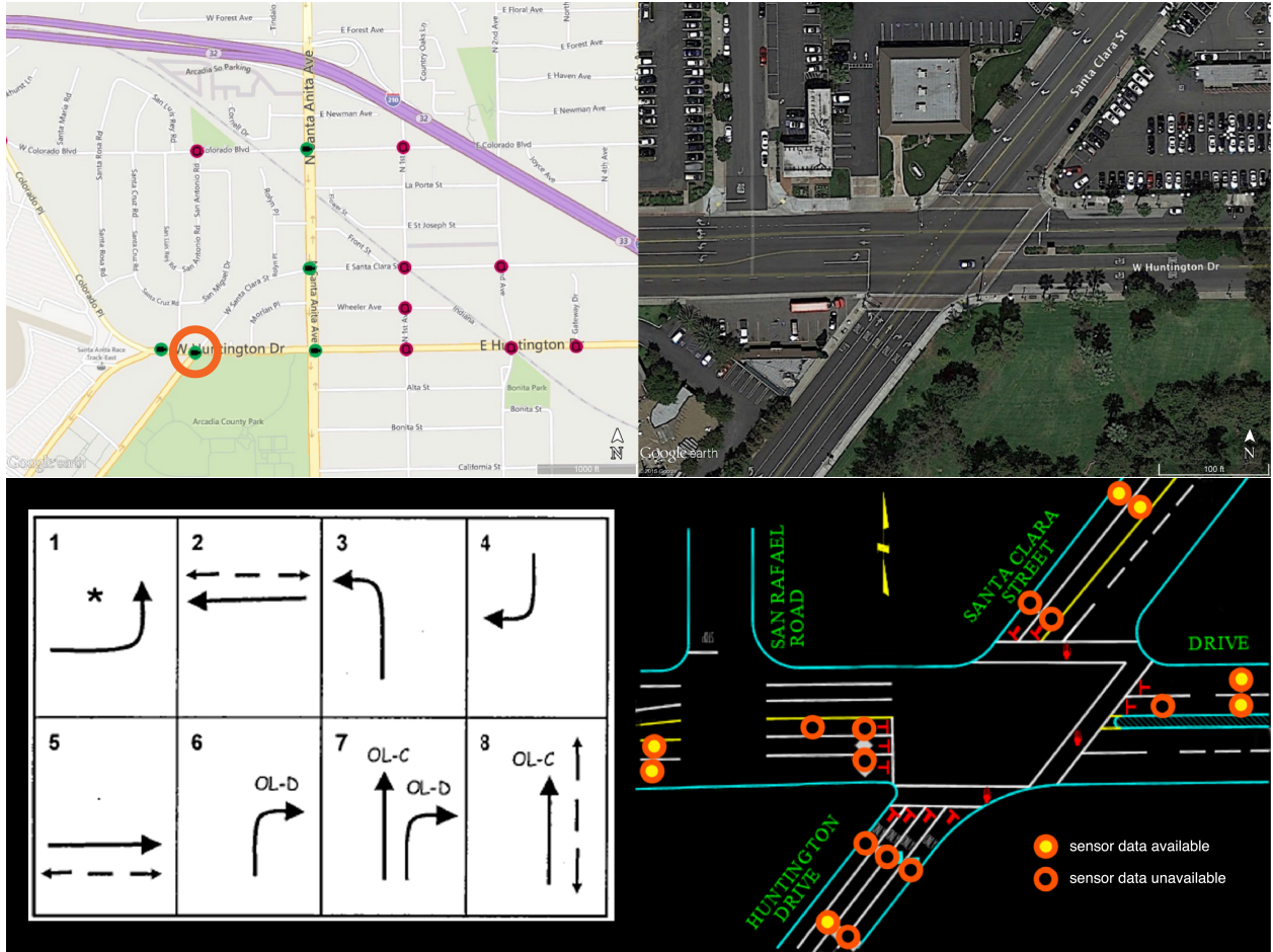
Figure 6.4: The intersection of Huntington Drive and Santa Clara Street in Arcadia, California has four approaches and three egresses. While sensors corresponding to each of the nine turning movements are installed, only data from seven approach sensors is collected centrally: measurements of north-bound right turns and north-bound left turns were not provided. Each sensor location returned 2 independent measurements: volume and time-occupancy. Thus there are a total of 14 measurements available for analysis.
