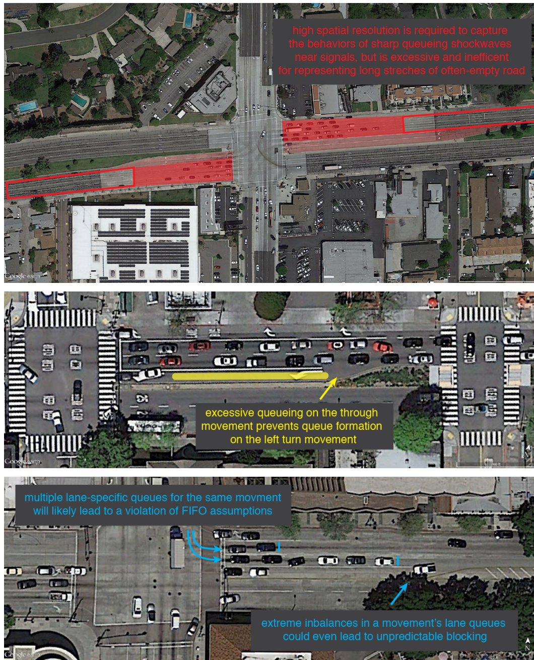
Figure 1.3: Many aspects of the queueing dynamics observed on signalized roadways make accurate modeling difficult. Sharp queueing shockwaves on signalized roadways would require excessive spatial discretization for accurate representation via CTM. Furthermore, a basic CTM is unable to model the interactions between movement-specific queues which form immediately upstream of a signalized intersection.
